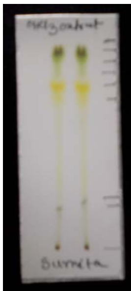
Fig. 2. TLC profile of the chloroform extract of N. nucifera leaf. Solvent system: benzene: chloroform: ethyl acetate (2: 3: 5). R_f values: 0.20, 0.24, 0.79, 0.77, 0.83, 0.88, 0.94
