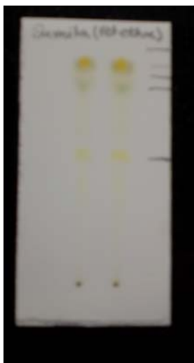
Fig. 1. TLC profile of the pet. ether extract of N. nucifera leaf. Solvent system: benzene: chloroform: ethyl acetate (5: 3: 2). R_f values: 0.54, 0.84, 0.89, 0.93.
