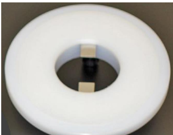
Figure 4. Shows colleactor (8) made from copper with electrode sharpe edges. 10mm * 20mm and thick ness 2mm a) Minus form b) with insulator on its sides.
