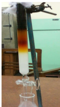
Figure-1: Column Chromatography of Petroleum spirit extract producing bands.
