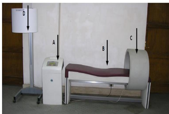
Figure 1: ASA magnetic field (Automatic PMT Quattro pro) A- The appliance, B- Motorized bed, C- Solenoid, D- Accessory for transcranial application
