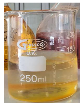
Figure 2. Yellow-orange precipitate obtained from titration of sulfide with cadmium
