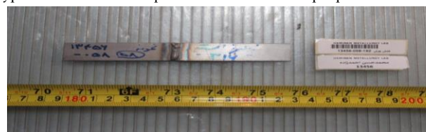
Figure 2. Inconel 617 using double-sided TIG welding with argon gas and 316 stainless steel filler
