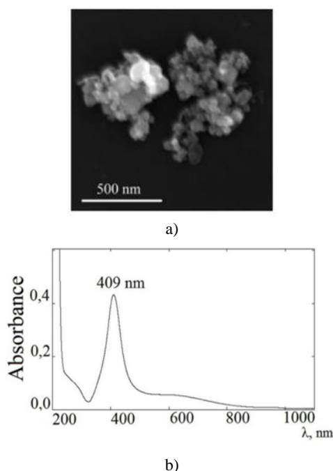
**Figure 1.** Characterization of silver nanoparticles: SEM micrographs (a) and absorption spectrum of UV-visible electromagnetic waves
